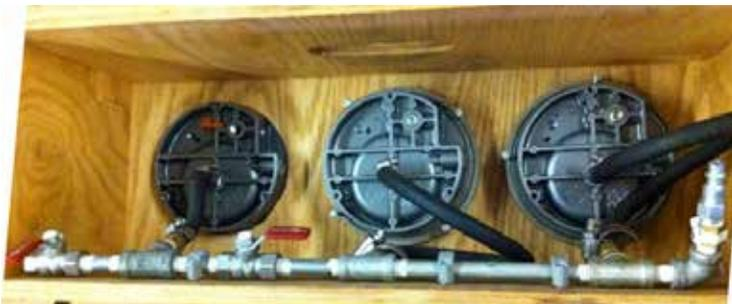
Inside my gauge kit I have plumbed the three gauges in series. By turning a valve, I can remove the 0-10 gauge from the series.
