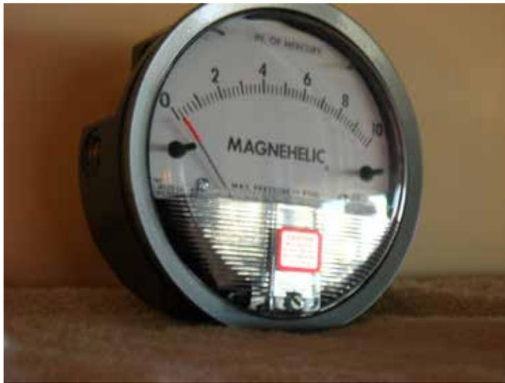
Gauges with a large face are easy to read. This one reads vacuum pressures from 0-10 inches Hg. It is easy to read small increments, like 5.1 inches Hg.
