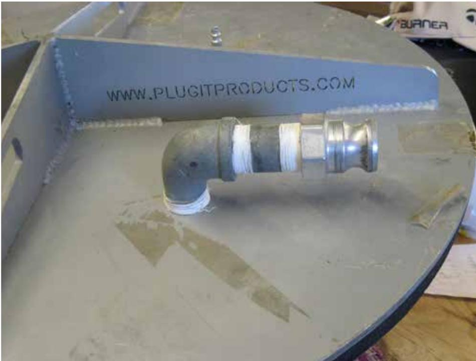
I have plumbed the top of the plate to receive the Cam-lock fitting on the end of the twenty foot hose. At top is a quick connect which I connect to my gauges by a 25 ft air hose. I stand away from tanks that are being tested at high pressures. Testing at 4 inches Hg for water tightness is not usually a danger, but I have imploded concrete tanks at 10 inches Hg. Mid-seam concrete tanks usually stand 13 inches Hg. top-seam tanks break at 8-10
