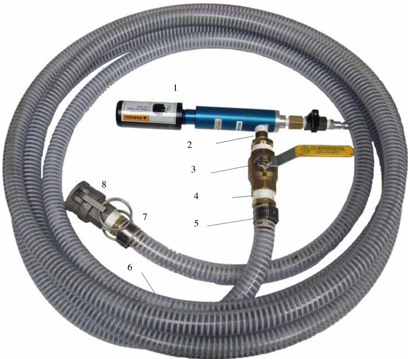
Venturi with hose. Allows tester to stand 20 ft away from test tank
