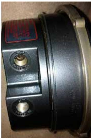
On the back and side of each gauge are two openings. One marked Low pressure and one marked "High pressure" Select which Low Pressure opening you are using, seal the other one with the provided plugs. Leave either one or both "High Pressure" Ports unplugged.
