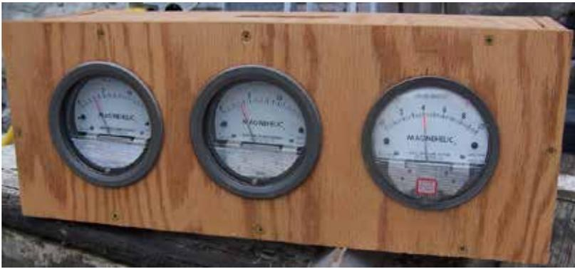
My gauge kit is home made, but effective. Two of the gauges read vacuum from 0-15 inches Hg. The other reads from 0-10. One verifies the others. I can disconnect the 0-10 gauge for elevated pressures.
