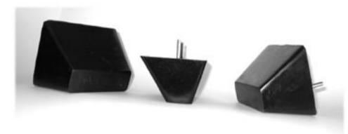
Molded of very tough polymers, these hole formers will last longer than any others. Deeply embedded ¼" studs are spaced at 45/6" centers. The extreme offset taper eases release.
