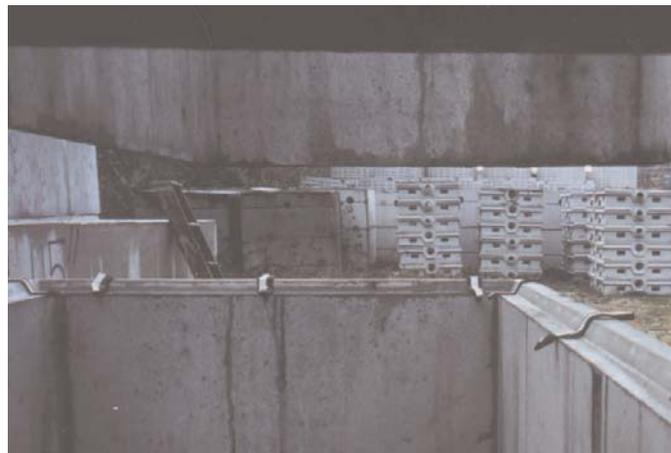
Bitewing test: Short strips of ConSeal placed across the joint are crushed when the top is assembled. The pattern of compression reveals the contour of the joint and what size sealant to use.
