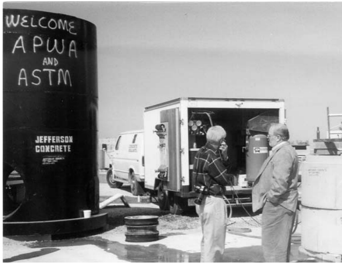
CONCRETE SEALANTS PROVIDES THEIR TESTING EQUIPMENT TO TEST JEFFERSON CONCRETE MANHOLES AND CONSEAL BUTYL
